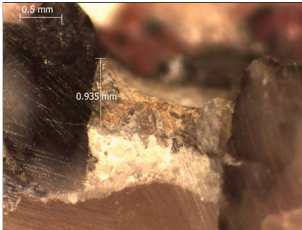
Figure 1. Inter-radicular perforation filled with material based on calcium aluminate. There is partial dissolution of the material, that is, disintegration with absorption of color and partial color change of the material ( \times 30 ).
