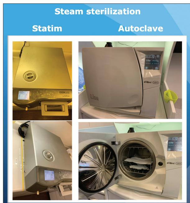
**Figure 4.** Steam sterilization: Statim and Autoclave
