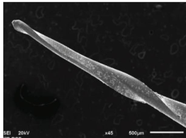
**Figure 6.** SE image of the apical segment of the Mtwo instrument (20/06 of the third group at magnification  $\times 45$ ) on which the straightening of the thread is observed
