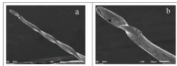
**Figure 5.** SE images: a) Mtwo instrument (10/04 of the second group at magnification  $\times 45$ ) on which changes in the thread (unscrewing, straightening) are observed; b) the apical segment of the Mtwo instrument (10/04 of the second group at magnification  $\times 150$ ) on which changes in the thread (unscrewing, straightening) are observed;
