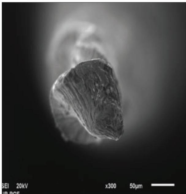
**Figure 7.** SE image of the fracture surface of the Mtwo instrument 15/05 at magnification  $\times 300$ , which shows a multitude of microfractures
