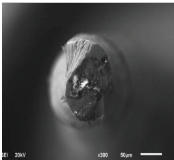
**Figure 2.** SE image of Mtwo 10/04 instrument with complete fracture (fractographic image at magnification  $\times 300$ ) which shows the difference in the appearance of the fracture surface in the central and peripheral area.
