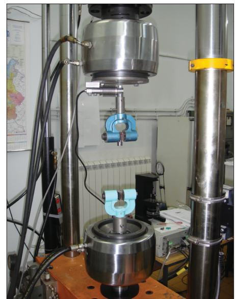
**Figure 2.** Universal testing machine with the clamps used to measure the separation force
