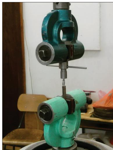
**Figure 3.** Detail of the universal testing machine just before the separation of metal cap from the abutment
