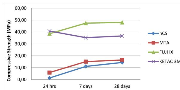
**Figure 1.** Compressive strength values (MPa) in the function of time
