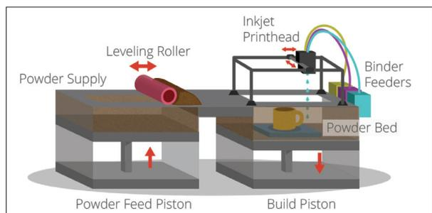
**Figure 7.** A binder is firstly jetted and selectively sprayed into a powder bed. When one layer is printed, the powder bed drops incrementally and a roller or blade applies and flattens the powder over the surface of the bed, prior to the next pass of the jet heads, with the binder for the subsequent layer to be formed and fused with the previous layer.
