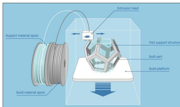
Figure 3. Scheme of fused deposition modelling technique (source: www.additively.com)
