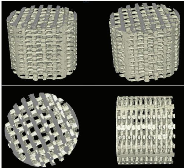
**Figure 4.** Micro CT volume reconstruction, example of porous bone scaffold structure, cylinder of 10 mm in height and 10 mm diameter. Cylinder is made by extrusion printing (FDM) and has ideal porosity, trabecular thickness, pore diameter and connectivity of pores for bone scaffold model.
