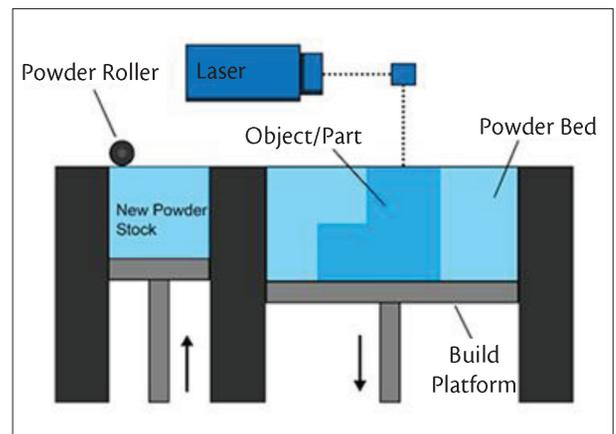
**Figure 2.** Powder Bed Fusion printer: A layer, typically 0.1mm thick material is spread over the built platform, then laser fuses the first layer or first cross section of the model. A new layer of powder is spread across the previous layer using a roller. Further layers or cross sections are fused and added. The process repeats until the entire model is created. Loose, un-fused powder remains in position but is removed during post processing.
